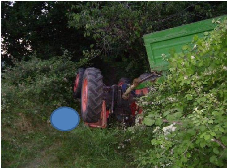
The operator was travelling with his agricultural tractor connected to a trailer. Due to a sudden depression of the ground the tractor rolled over and the operator remained crushed beneath it.
