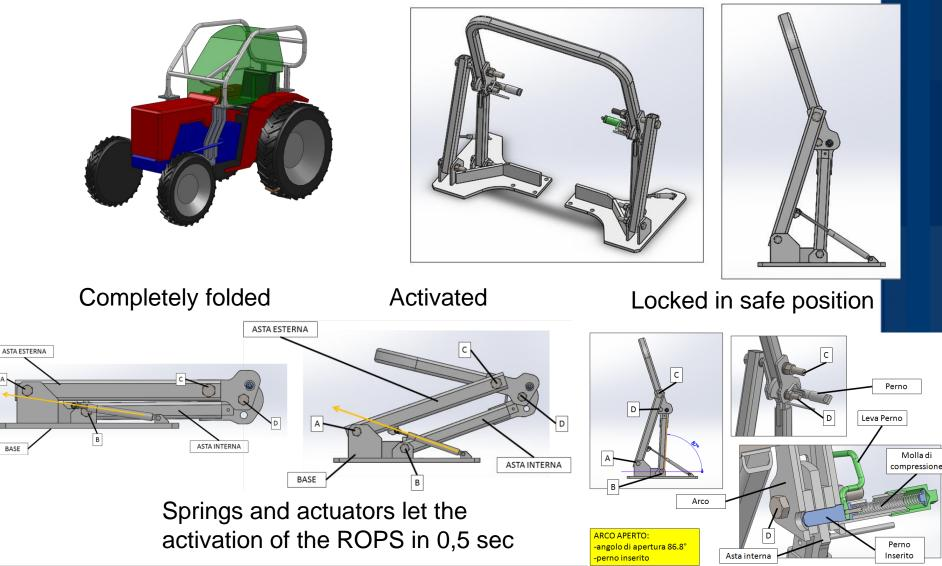
Design of Compact Tractor with reduced overall height.
