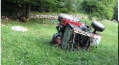
While working with tractor in the field he lost the control sliding on the grass and rolling over three times.
