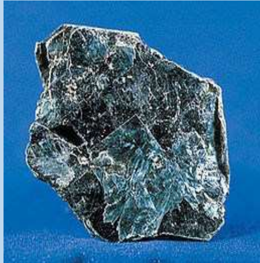
Vermiculite (\text{Mg}, \text{Fe}^{++}, \text{Al})_3(\text{Al}, \text{Si})_4\text{O}_{10}(\text{OH})_2 \cdot 4(\text{H}_2\text{O}) Simmetria Monoclino, cristalli tabulari, lamellari
